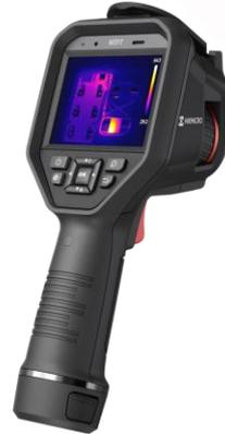
The HIKMICRO M31T handheld thermal imaging camera is engineered for high-precision temperature monitoring within critical ranges. Equipped with a 384×288 resolution, advanced calibration algorithms, it enables rapid identification of temperature anomalies in dynamic environments. With real-time temperature tracking at  $\pm 0.5^{\circ}\text{C}$  accuracy (ambient temperature:  $5^{\circ}\text{C}$ – $40^{\circ}\text{C}$ ), the device supports informed decision-making and enhances safety.
